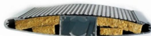
The blade encapsulates noise absorbing fibreglass. The padding is additionally covered with a black fibreglass tissue.
