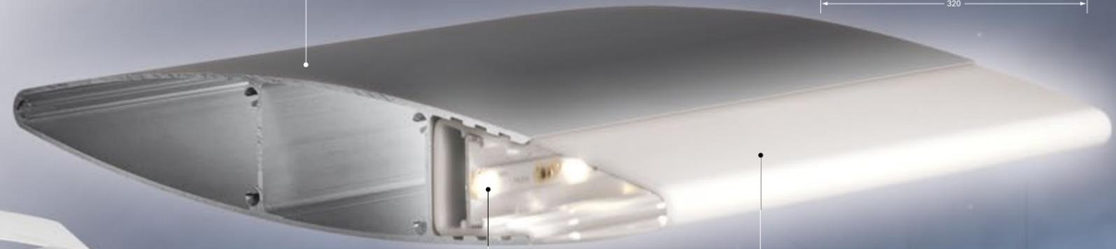
● **Blade profiles:** c|sairfoil LUX® illuminated blades are manufactured from extruded aluminium profiles in widths of 200 mm and 320 mm and can be shipped powder-coated in all available RAL-colours.
